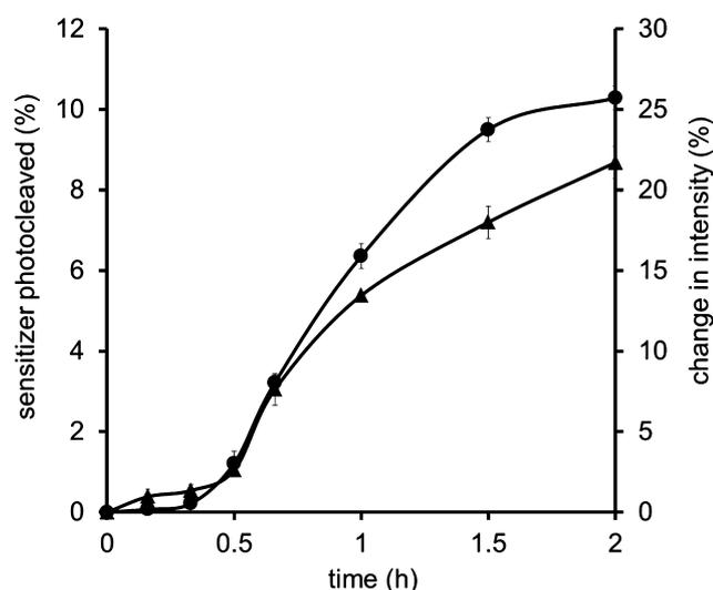
**Figure 3.** A time-sequence analysis of pheophorbide photoreleased free from the probe tip of the device in PBS at 25°C (solid circles) and fluence from the tip (solid triangles). The concentration of pheophorbide was measured by fluorescence spectroscopy at the indicated times. The values shown here are an average of 3 or more measurements.
