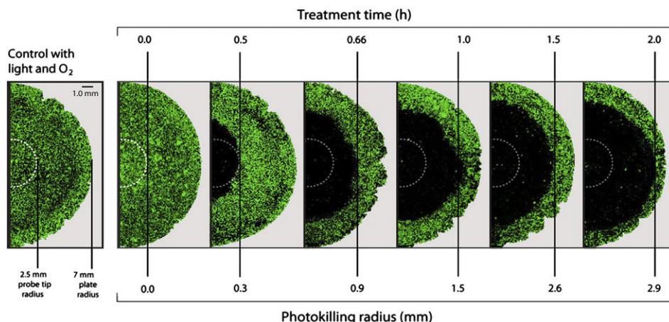
**Figure 5.** Device tip treatment of a U87 cell monolayer (154  $\text{mm}^2$  area) revealed a radius of photokilling as a function of time. Regions of the confocal fluorescence images show the probe tip radius in a white dashed line, the radius of photokilling and that of the plate edge. The cells were stained with calcein AM (green/live) for 30 min. Magnification 10 $\times$ .
