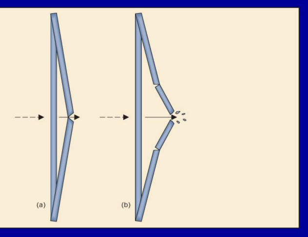
Production of radial and concentric fractures in glass. (a) Radial cracks are formed first, commencing on the side of the glass opposite to the destructive force. (b) Concentric cracks occur afterward, starting on the same side as the force.
