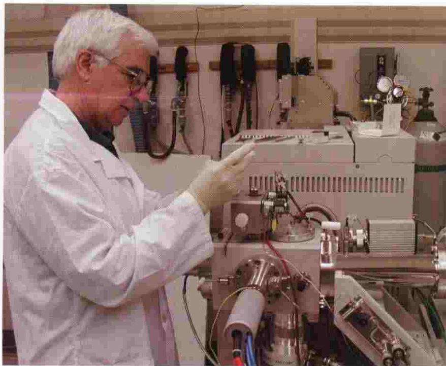
Figure 5. At its Environmental Health Laboratory, CDC scientists use several types of high-resolution mass spectrometry to analyze human tissue and fluid samples. The equipment shown here is being used to measure dioxin levels in a sample of blood serum. (Photograph courtesy of James L. Pirkle.)
