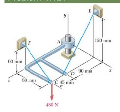
The assembly shown is welded to collar A that fits on the vertical pin shown. The pin can exert couples about the x and z axes but does not prevent motion about or along the y axis. For the loading shown, determine the tension in each cable and the reaction at A.
