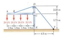
The frame shown supports part of the roof of a small building. Your goal is to draw the free body diagram (FBD) for the frame. (Neglect the weight of objects.)
