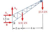
• Determine  $B \sum M_A = 0: +B(1.5\text{m}) - 9.81 \text{ kN}(2\text{m})$
