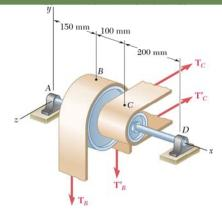
Two transmission belts pass over a double-sheaved pulley that is attached to an axle supported by bearings at *A* and *D*. The radius of the inner sheave is 125 mm and the radius of the outer sheave is 250 mm. Knowing that when the system is at rest, the tension is 90 N in both portions of belt *B* and 150 N in both portions of belt *C*, determine the reactions at *A* and *D*. Assume that the bearing at *D* does not exert any axial thrust.
