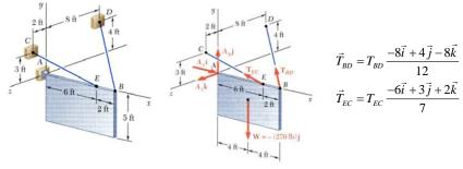
A sign of uniform density weighs 270 lb and is supported by a ball-and-socket joint at *A* and by two cables.
