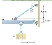
A 50-kg crate is attached to the trolley-beam system shown. Knowing that a = 1.5 m, determine (a) the tension in cable CD, (b) the reaction at B.
