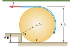
A 500-lb cylindrical tank, 8 ft in diameter, is to be raised over a 2ft obstruction. A cable is wrapped around the tank and pulled horizontally as shown. Knowing that the corner of the obstruction at A is rough, find the required tension in the cable and the reaction at A.
