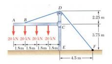
The frame supports part of the roof of a small building. The tension in the cable is 150 kN.
