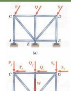
• Equal number unknowns and equations but improperly constrained
