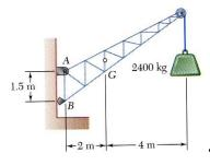
A fixed crane has a mass of 1000 kg and is used to lift a 2400 kg crate. It is held in place by a pin at A and a rocker at B. The center of gravity of the crane is located at *G*.
