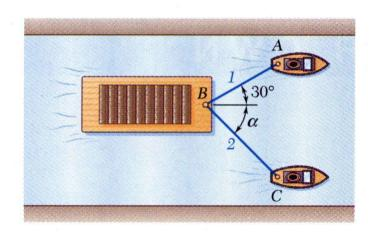
A barge is pulled by two tugboats. If the resultant of the forces exerted by the tugboats is 5000 lbf directed along the axis of the barge, determine the tension in each of the ropes for  $\alpha = 45^{\circ}$ .
