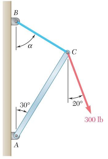
Knowing that  $\alpha = 55^{\circ}$  and that boom AC exerts on pin C a force directed along line AC, determine (a) the magnitude of that force (b) the tension in cable BC.
