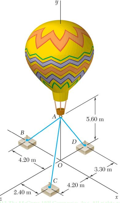
Three cables are used to tether a balloon as shown. Determine the vertical force **P** exerted by the balloon at *A* knowing that the tension in cable *AD* is 481 N.
