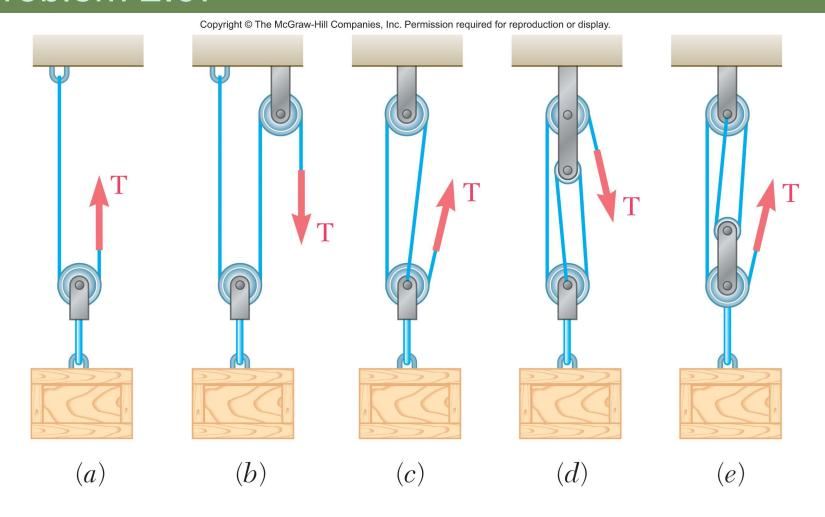
A 600-lb crate is supported by several rope-and-pulley arrangements as shown. Determine for each arrangement the tension in the rope.
