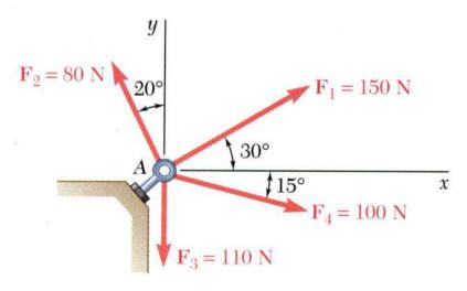
Four forces act on bolt A as shown. Determine the resultant of the force on the bolt.
