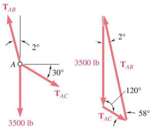
In a ship-unloading operation, a 3500-lb automobile is supported by a cable. A rope is tied to the cable and pulled to center the automobile over its intended position. What is the tension in the rope?
