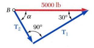
• The minimum tension in rope 2 occurs when  $T_1$  and  $T_2$  are perpendicular.
