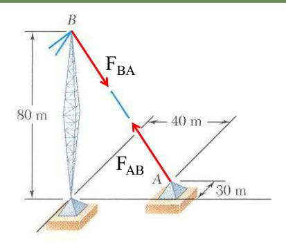
What are the components of the force in the wire at point B? Can you find it without doing any calculations?
