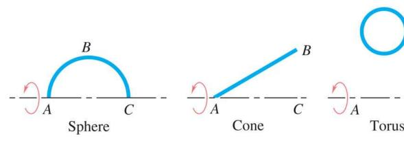
• Surface of revolution is generated by rotating a plane curve about a fixed axis.
