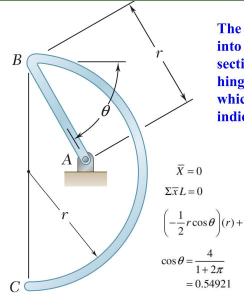
The homogeneous wire *ABC* is bent into a semicircular arc and a straight section as shown and is attached to a hinge at *A*. Determine the value of  $\theta$  for which the wire is in equilibrium for the indicated position.
