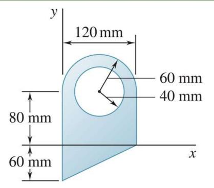
For the plane area shown, determine the first moments with respect to the x and y axes and the location of the centroid.
