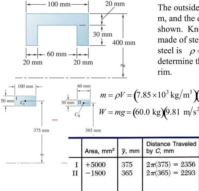
The outside diameter of a pulley is 0.8 m, and the cross section of its rim is as shown. Knowing that the pulley is made of steel and that the density of steel is  $\rho = 7.85 \times 10^3 \text{ kg/m}^3$ determine the mass and weight of the
