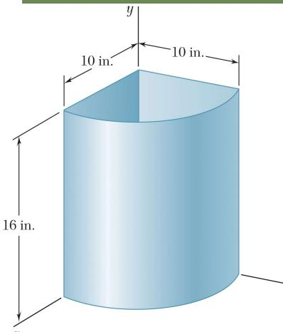
A wastebasket, designed to fit in the corner of a room, is 16 in. high and has a base in the shape of a quarter circle of radius 10 in. Locate the center of gravity of the wastebasket, knowing that it is made of sheet metal of uniform thickness.
