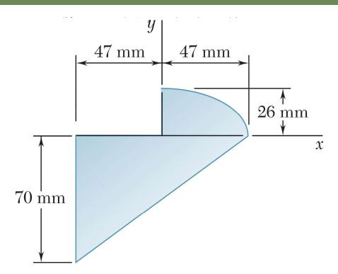
Determine by direct integration the centroid of the area shown. Express your answer in terms of *a* and *b*. Locate the centroid of the plane area, which consists of a quarterellipse and a triangle.
